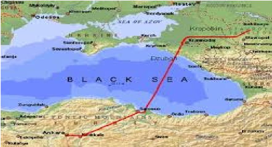
The Blue Stream gas pipeline is designed to supply Russian gas directly to Turkey via the Black Sea.
